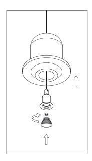
Lift the onyx part and insert the GU10 bulb. Warning: Use only LED
