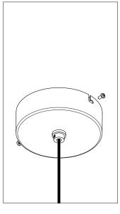
Fix the ceiling rose with the screws on the mounting plate.
