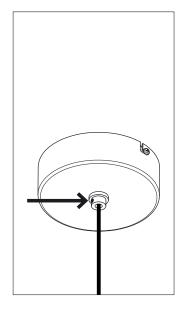
4 Secure the fixing screw.
