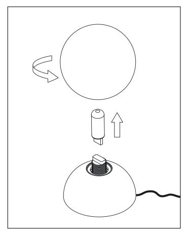
1 Unscrew the glass sphere from the socket. Insert the G9 bulb. Screw the glass sphere onto the socket. Take care to screw the glass sphere gently. **Warning:** Use only LED
