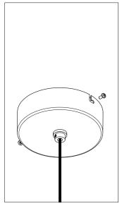
3 Fix the ceiling rose with the screws on the mounting plate.
