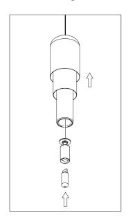
Lift the brass and glass parts. Insert the G9 bulb. Warning: Use only LED
