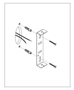
Disconnect the power by turning off the circuit breaker, or by removing the fuse in the fuse box before assembling and mounting the canopy. Fix the mounting plate to the ceiling with dowels and screws.
