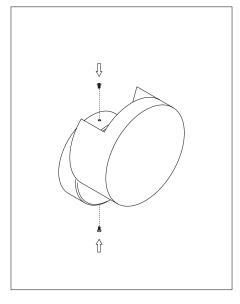
Fix the ceiling rose with the screws on the mounting plate
